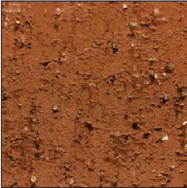
1 BRICK VENEER & ROWLOCK: SUMMIT BRICK COLOR: WIRE-CUT RED(4-212)
